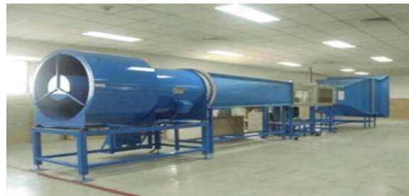
Fig. 6: Wind tunnel used for experiments
