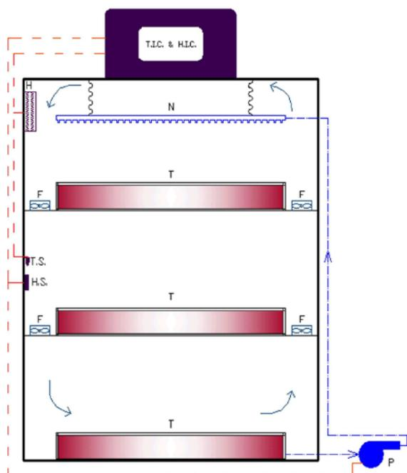
Fig. 1: Schematic diagram of the tray bioreactor set up;
