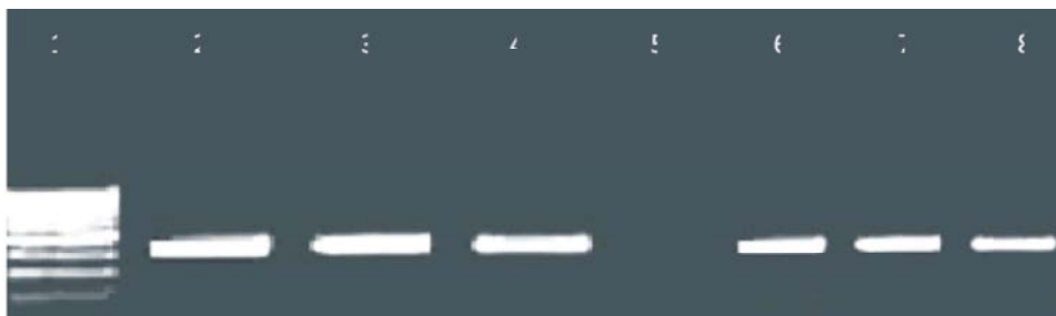
Fig. 3: Amplified PPR after agarose gel electrophoresis, ethidium bromide staining and UV trans-illumination. Lane 1, contain 100bp marker while lane 2, 3, 4, 6, 7 contain PPR where an illuminating band at 350bp. Lane 8 contain control positive
