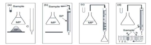
Fig. 1: (a) Components (C: column; SP: stationary phase; MP: movement phase; Sample: mare's milk whey (b) the process of putting the sample into the column (c) the proses of elution (d) isolation sample.
