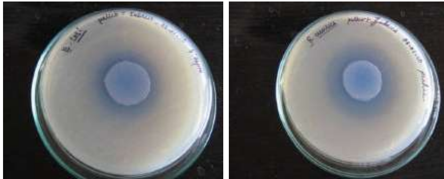
Fig. 1: Antibacterial activity of Pellet containing \text{CuSO}_4 finished fabric against staphylococcus aureus and Escherichia coli
