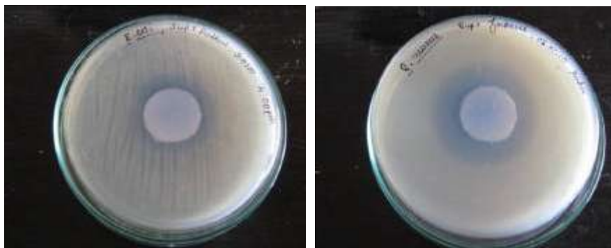
Fig. 2: Antibacterial activity of supernatant containing \text{CuSO}_4 finished fabric against staphylococcus aureus and Escherichia coli
