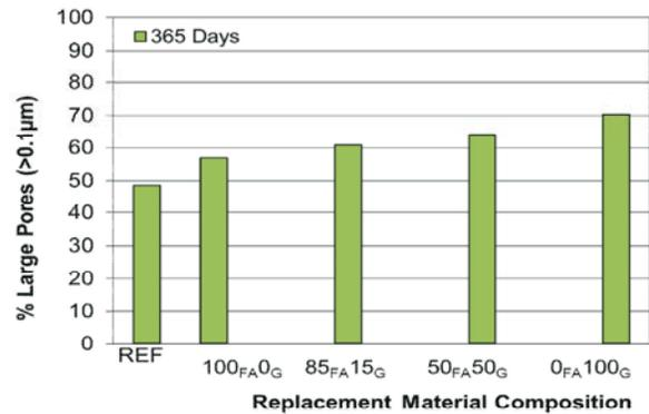
Fig. 8: Influence of FA-G composition on the percentage of large pores (>0.1 µm) of pastes
