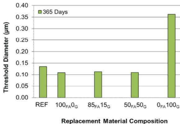
Fig. 7: Influence of FA-G composition on the threshold diameter (TD) of pastes
