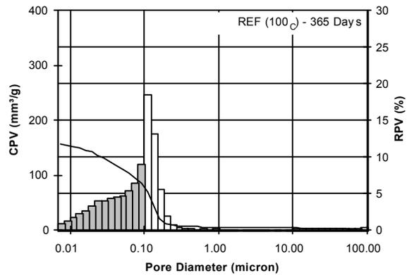
Fig. 2: Pore size distribution of the reference paste (M1)
