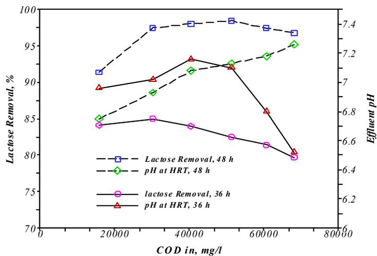
Fig. 6: Lactose conversion and effluent pH
