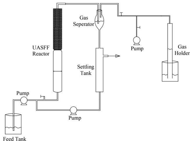
Fig. 1: Schematic diagram of the UASFF bioreactor
