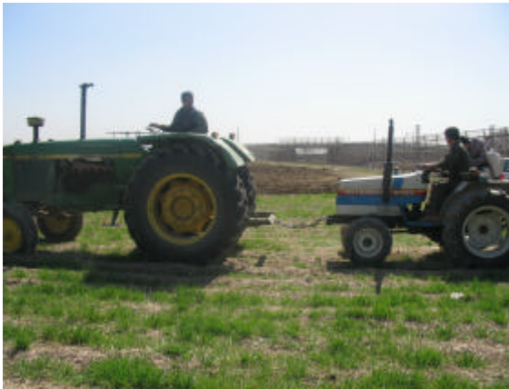
Fig. 4: Field tests for measurement of slip and tractive force
