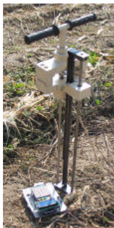
Fig. 2: Digital hand-pushed penetrometer
