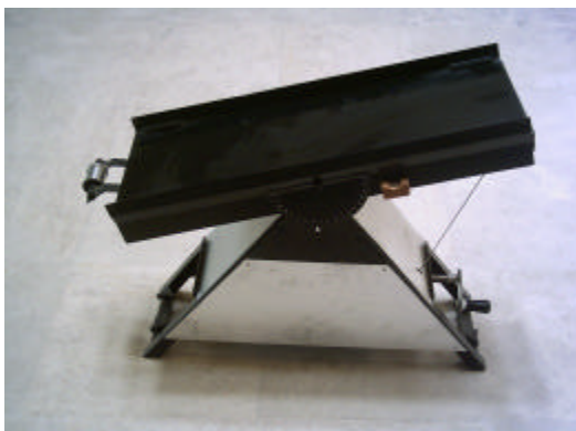
Fig. 2: Apparatus to determine static coefficient of friction
