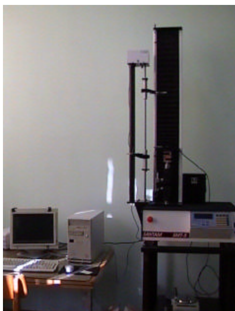
Fig. 4: A universal testing machine (Santam, MRT-5) to determine failure properties of fruits
