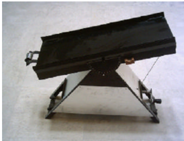
Fig. 3: Apparatus for measuring static coefficient of friction
