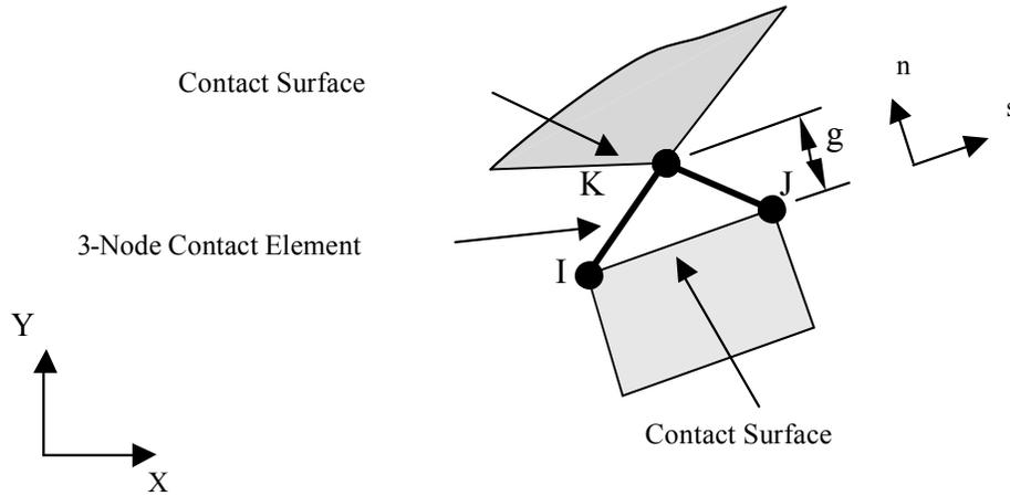
Fig. 4. The geometry of 3-node contact element
