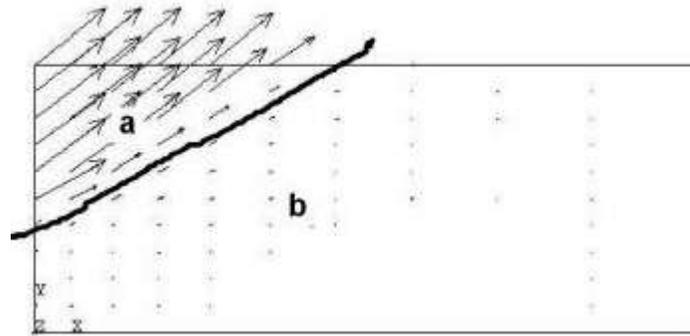
Fig. 6: Soil node displacement vectors
