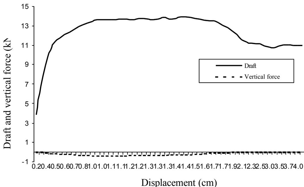
Fig. 5: Draft force (up) and vertical force (down) acting on the blade vs. displacement
