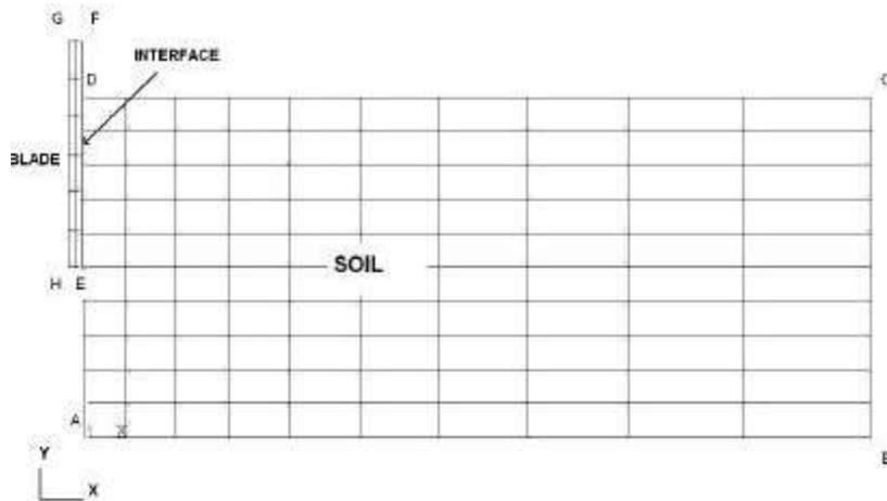
Fig. 3: The 2D meshing of soil-blade and boundary conditions
