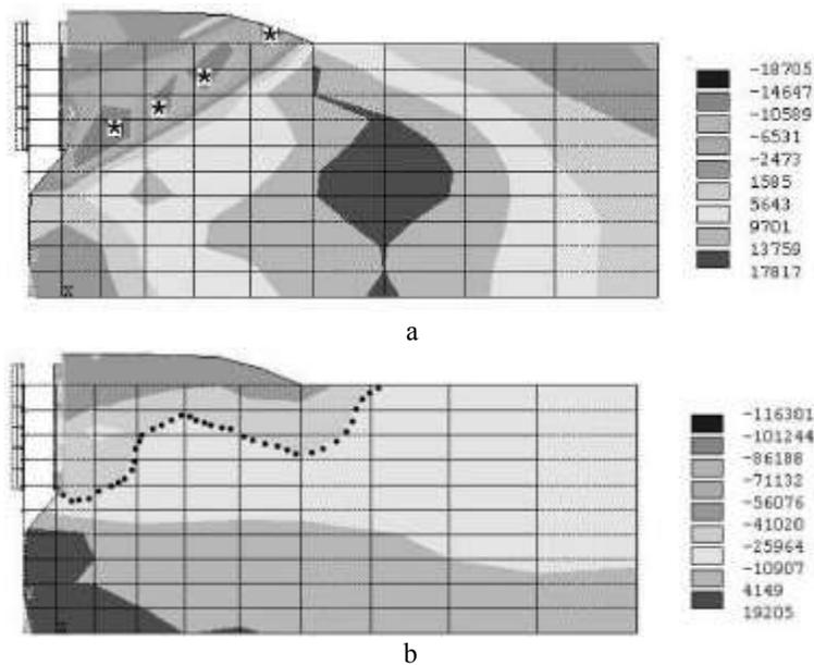
Fig. 7: a) Shear stress in the soil. The maximum absolute shear stress value is shown by "\*". b) Minor principal stresses. The failure edge due to tensile is shown by "..."
