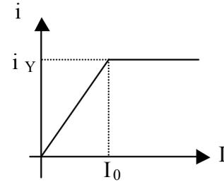
Fig. 1: Stress-strain behaviour of elastic-perfectly plastic soil
