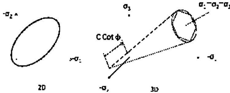
Fig. 2: Drucker-Prager's yield surface in 2D space (left) and 3D space (right)
