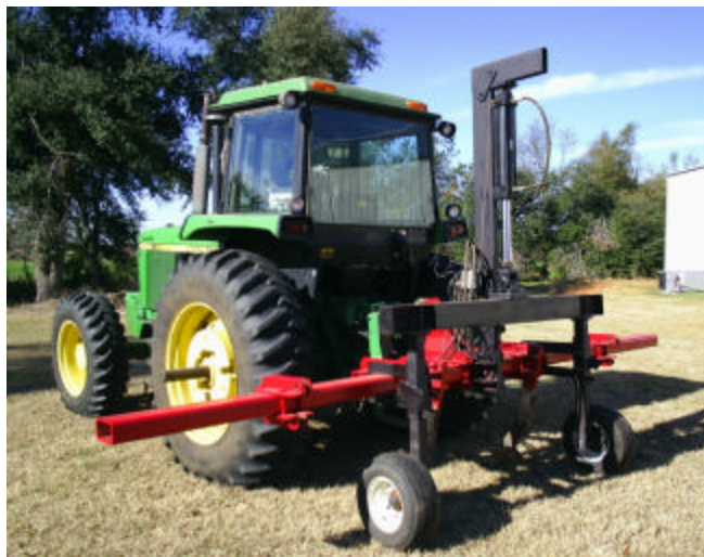
Fig. 2: The control system for variable-depth tillage operations
