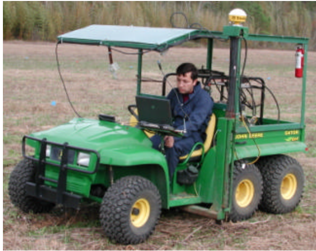
Fig. 1: Hydraulically operated penetrometer system with DGPS unit
