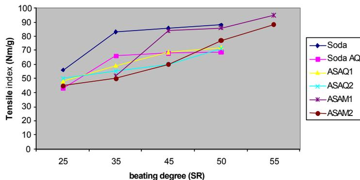
Fig. 1: Tensile index for different beating degrees of unbleached *Cajanus cajan* Pulps
