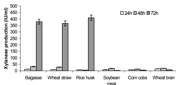
Fig. 8: Production of xylanase by Bacillus subtilis -BS05 using media-IV under static conditions at 37°C. Bars represent the standard deviation among replicates which differ significantly at p \leq 0.05
